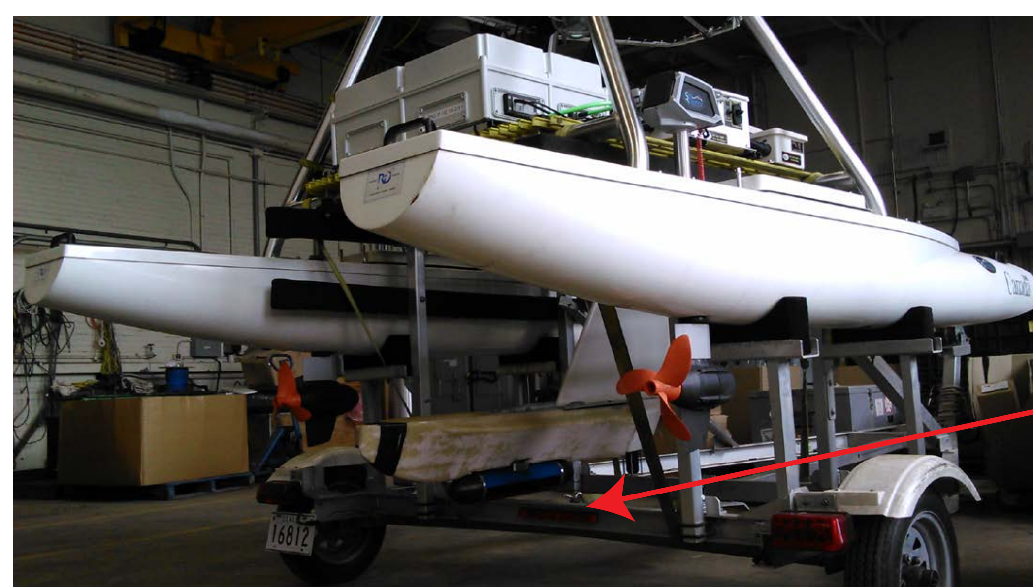
Sea Robotics USV-2600 4-m catamaran unmanned surface vehicle, with sonar installed at bottom of keel
