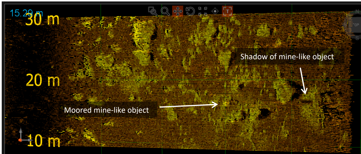
Figure 1: Geometrically correct 3D Sidescan viewed from directly overhead and colored by backscatter intensity.
