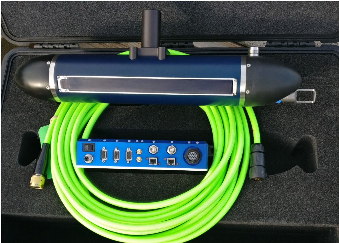
Figure 1: 3DSS-iDX-450 Sonar with new Sonar Interface Unit
